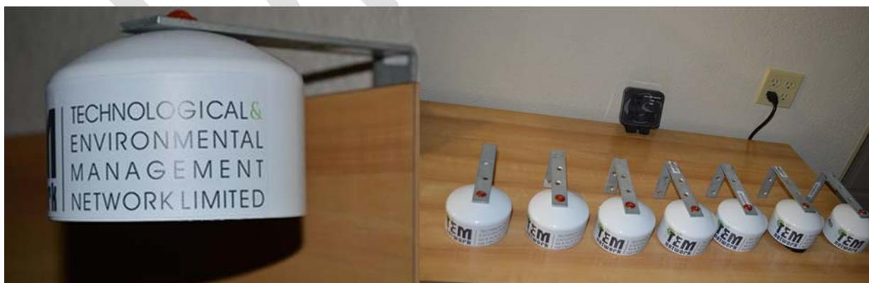
Figure 2: PSD custom-build rain shelter.
