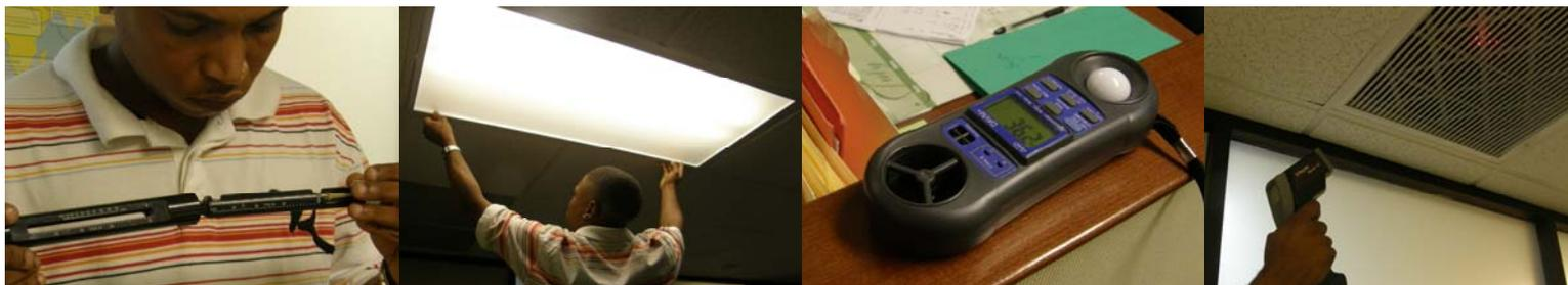
Left to right, Mr. Chaz measures humidity levels, inspects lights installed, records light levels using a light meter and measures temperatures emitted from the A/C vents
