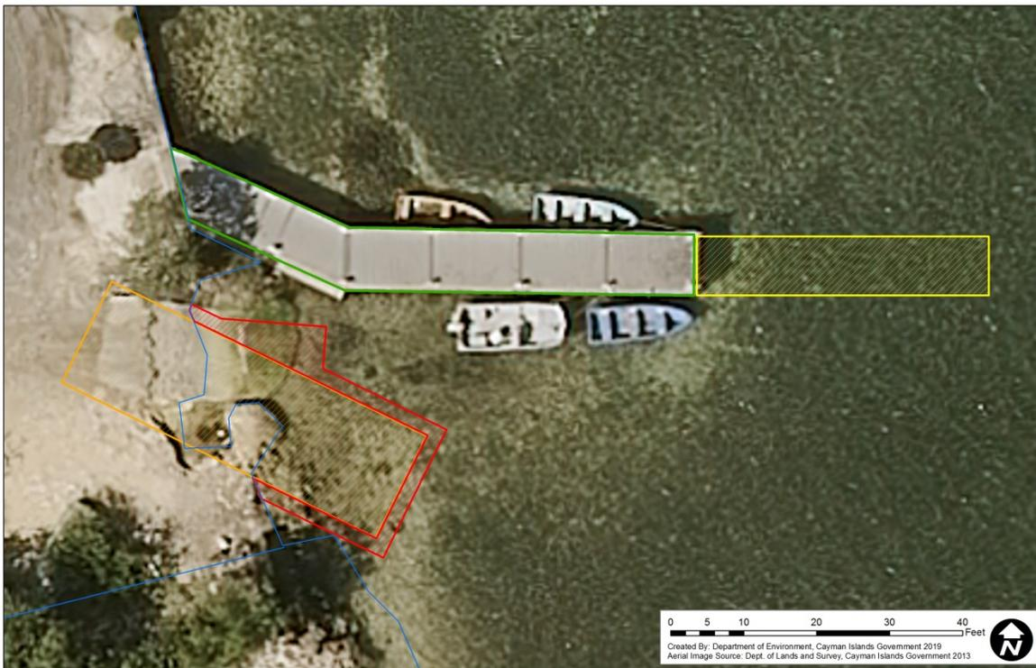
Figure 1: 2013 LIS aerial imagery showing proposed dock renovation area (green) extension (yellow), boat ramp removal and excavation area (red) and new boat ramp area (orange) (LIS 2013, DOE 2019)
