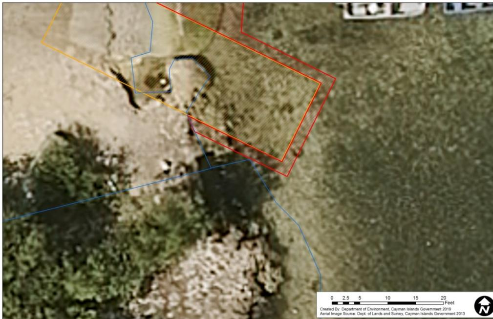
Figure 3: 2013 LIS aerial imagery showing proposed excavation area (red) and new boat ramp area (orange), and the alignment with the MHW and parcel boundary (blue) (LIS 2013, DOE 2019)
