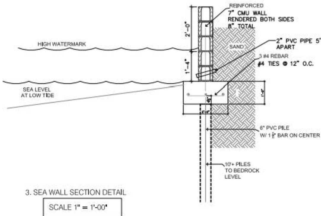
**FIGURE 3: EXTRACT FROM APPLICANT'S SUBMISSIONS SHOWING THE CROSS SECTION OF THE PROPOSED SEA WALL. (SOURCE: ARCO, 10 OCTOBER, 2021)**
